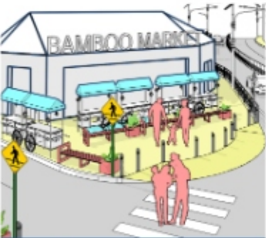
Figure 3.28 Footpath extended at junction corners Source: WRI India
