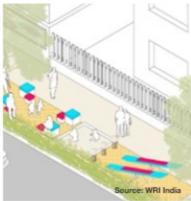
Figure 3.53 Minimum of 2 metre wide footpaths
