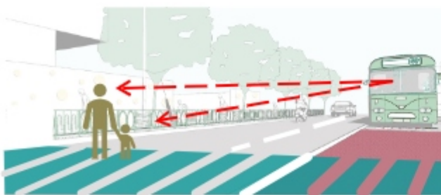
Figure 3.27 Visibility at pedestrian crossing Source: WRI India
