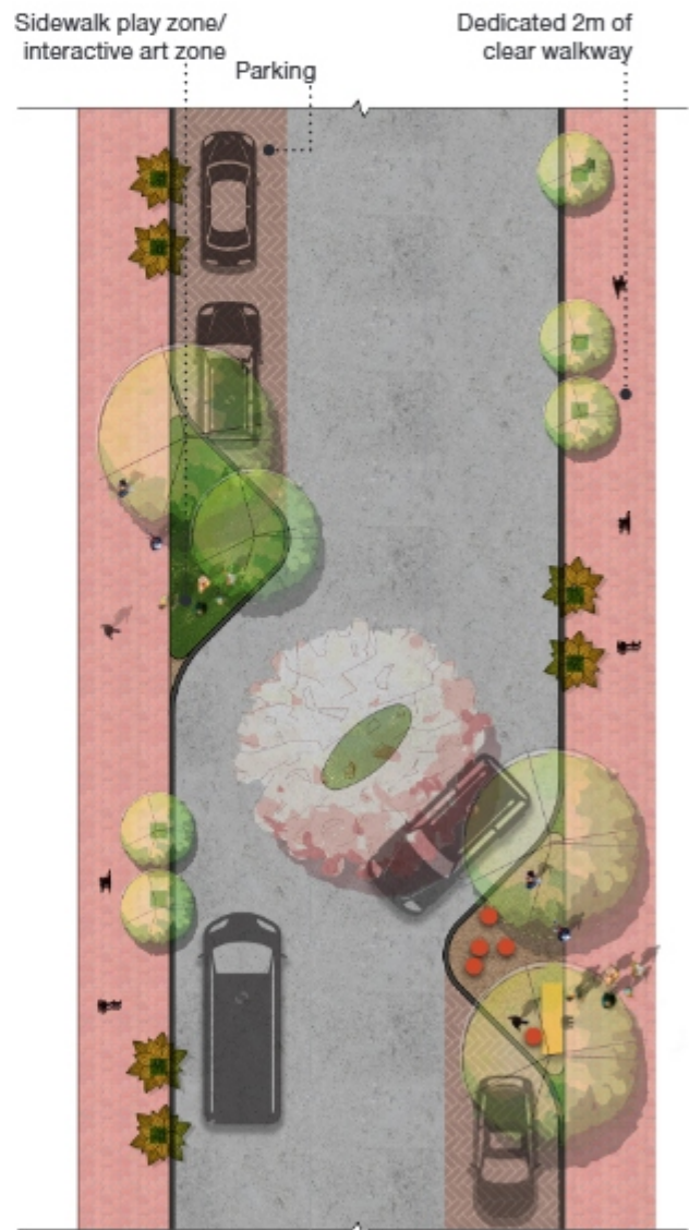
Figure 3.22 12 metre chicane street section and plan
