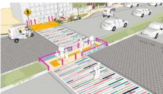
Figure 3.29 Wider refuge median with staggered crossing Source: WRI India
